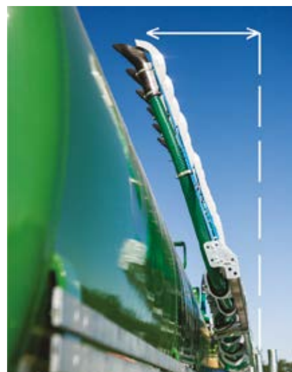
Springs are positioned to the inside in transport position
