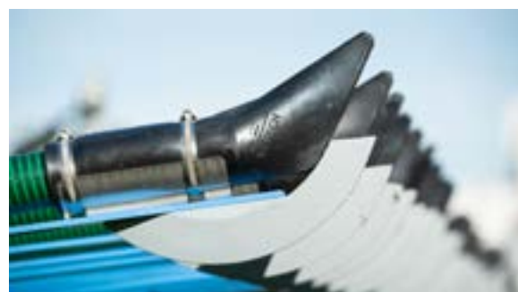
Specially designed trailing shoe
